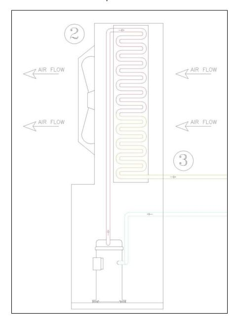
The latent heat required to condense this gas is rejected from the refrigerant into the outside air. This process is called condensation, thus the coil which this occurs is referred to as the condenser. The temperature that the condensation occurs is much higher than within the evaporator, as the pressures in the condenser are much higher.
