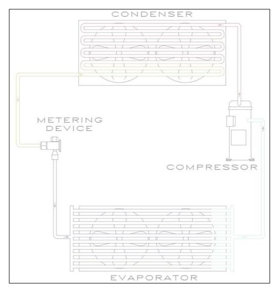
Most of the heat transfer occurs because the refrigerant changes state. The liquid refrigerant in the evaporator absorbs its latent heat of vaporization, and in the process changes from a liquid to a vapor. The gas refrigerant within the condenser rejects its latent heat of vaporization, thus changing from a gas to a liquid. It is this cycle change that moves the removed heat from one place to another.
