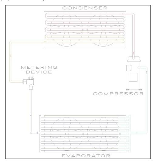
What is Refrigeration? Refrigeration is simply cooling by removing heat. Heat is a form of energy that can't be destroyed. Therefore to remove heat we can only transfer from one place to another. Even though it is easier to think of refrigeration as the process of making things cold, it actually is the process of transferring heat from one place to another.
