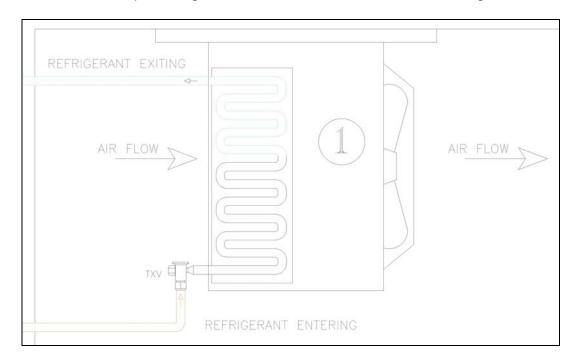
The Latent heat required to boil off this refrigerant from a liquid to a gas is taken from the air as it passes through the coil, thus cooling the air. This boiling process is called evaporation, thus the coil in which this occurs is referred to as our Evaporator. The Evaporator is where we collect the heat we want to remove.
