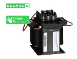
Industrial control transformer, Type TF, 1 phase, 500VA, 208/230/460V primary, 115V secondary, 50/60Hz
